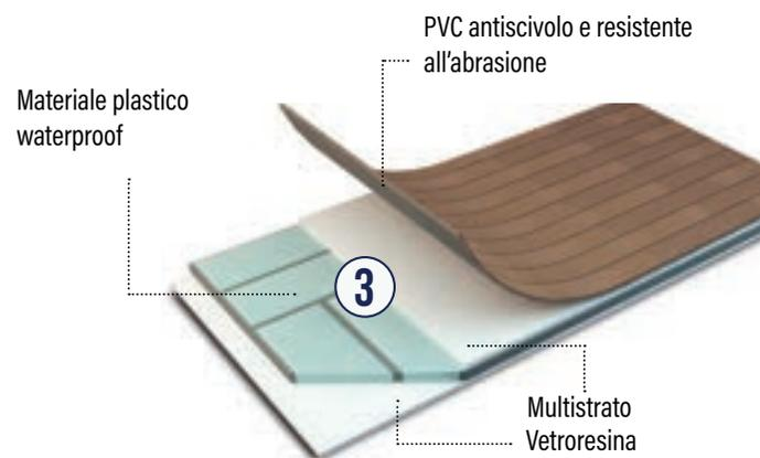
**PAVIMENTO** DI 54 MM DI SPESSORE, CON RIVESTIMENTO INTERNO IN PVC ANTISCIVOLO RESISTENTE ALL'ABRASIONE, COSTITUITO DA UNA LASTRA IN VETRORESINA ESTERNA E MULTISTRATO INTERNO, TELAIO IN PVC E INSERTI IN MATERIALE PLASTICO WATERPROOF.
