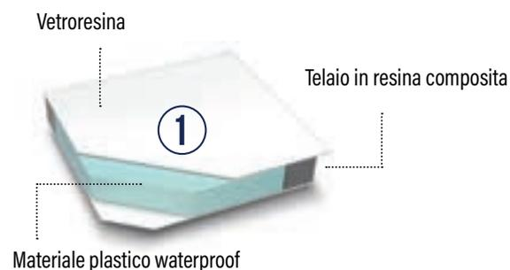
**TETTO** FORMATO DA UNA DOPPIA LASTRA DI VETRORESINA, ESTERNA ED INTERNA, TELAIO IN PVC E INSERTI DI MATERIALE PLASTICO WATERPROOF, SPESSORE DI 30 MM.
